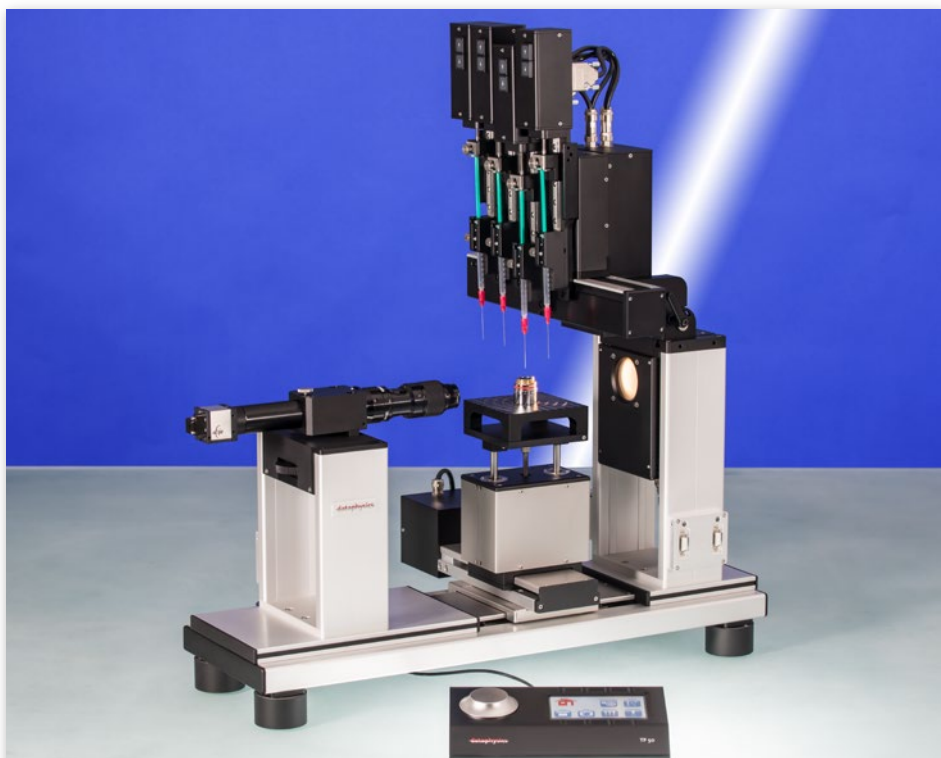
OCA 50 with a fourfold electronic direct dosing system DDE/4, four electronic syringe modules ESr and TP 50 control panel
