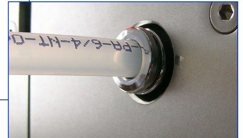
External gas supply at HGC 30
