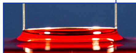
determination of the surface tension using a Du Noüy ring
