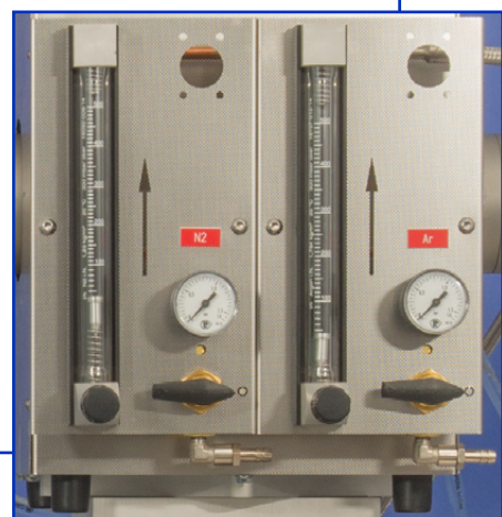
gas supply system
