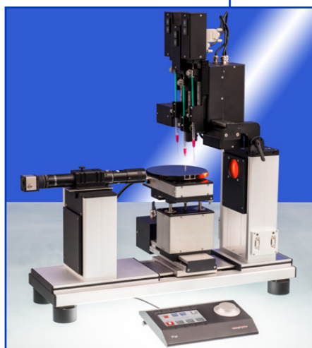
Analysis of the surface free energy by fully automatic wafer mapping
