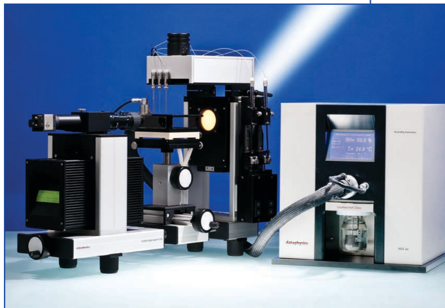
Humidity Generator and Controller HGC 20 connected to the TPC 160 of an OCA 20
